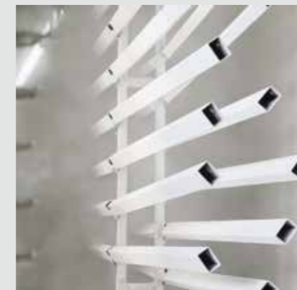
The level of powder coating amounts to 80 - 100 µm, subsequent curing at 180°C in the oven
