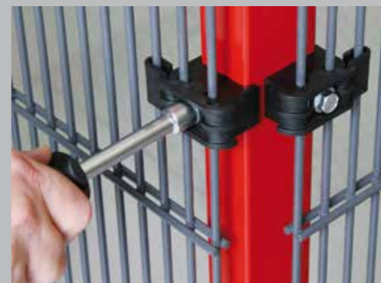
A tool must be required to open up the fixing elements of the protective fence.
