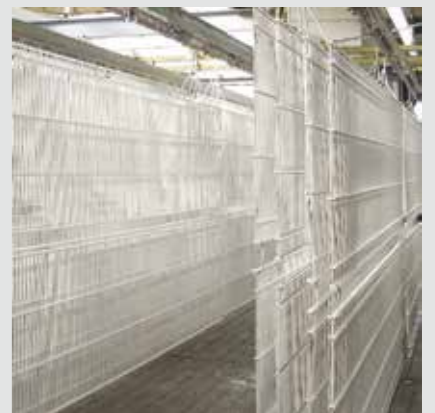
After a cooling period the mesh sheets are ready for shipping
