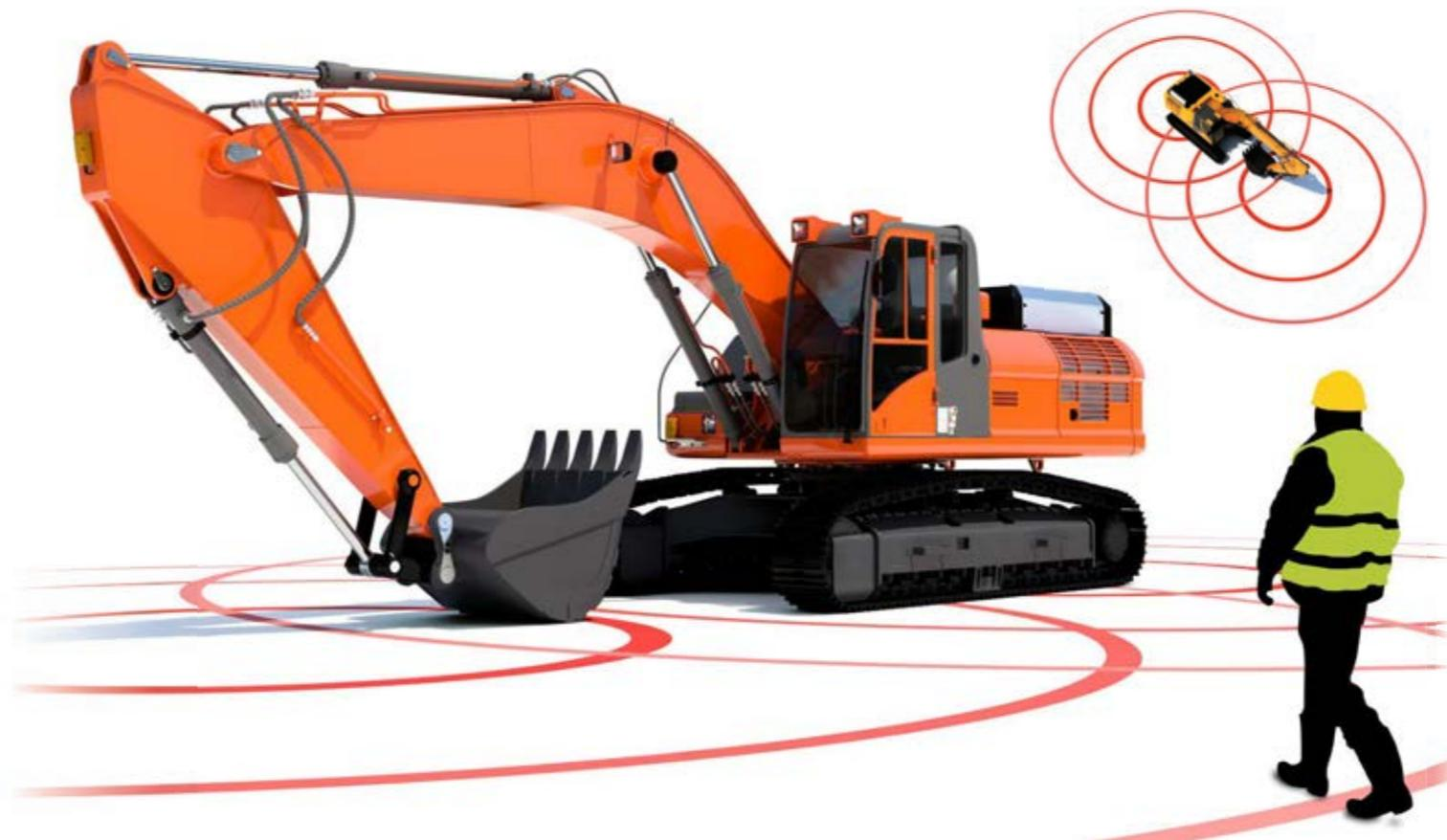
An excavator can be fitted with multiple detection zones to cover key areas of the machine including rear slewing area, operator blind zones and arm or bucket.
