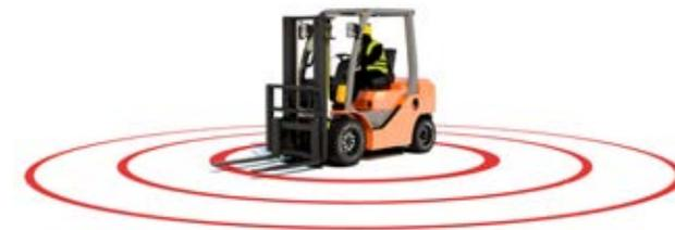
Single Zone Detection - most commonly used on forklift trucks and small plant.
