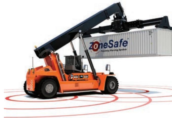
Large vehicles such as reach stackers can be fitted with multiple detection zones to cover key areas of the machine including the rear turning area, blind zones and spreaders.
