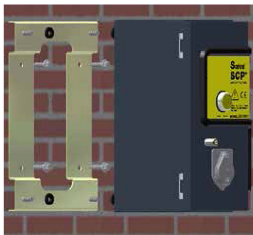
Typical SCP+ installation location using mounting plate.
